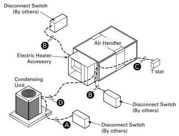
Figure 21. Field Wiring Outdoor/Indoor
